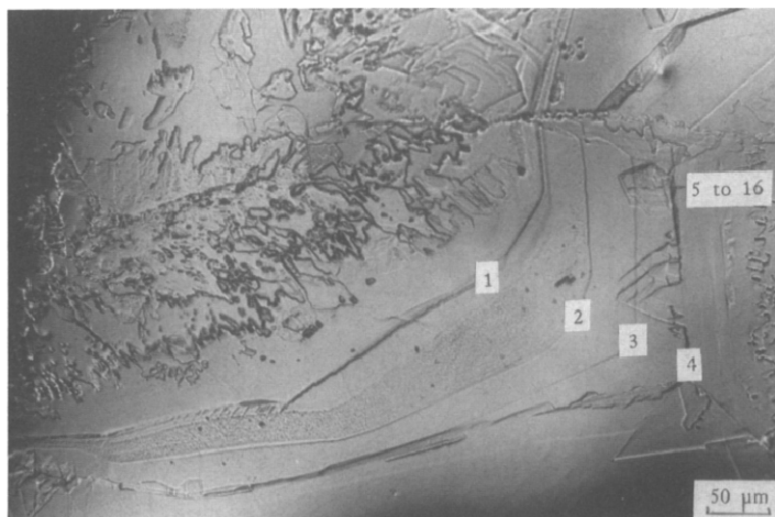
Fig. 5. Alloy 793 (Pb-0.093wt.%Ca). First and second discontinuous transformations. Apparent rate of boundary movement: 10\ \mu\text{m} and 1\ \mu\text{m}\ \text{min}^{-1} for first and second transformations, respectively. 16 etchings with \Delta t = 2\ \text{min} .
